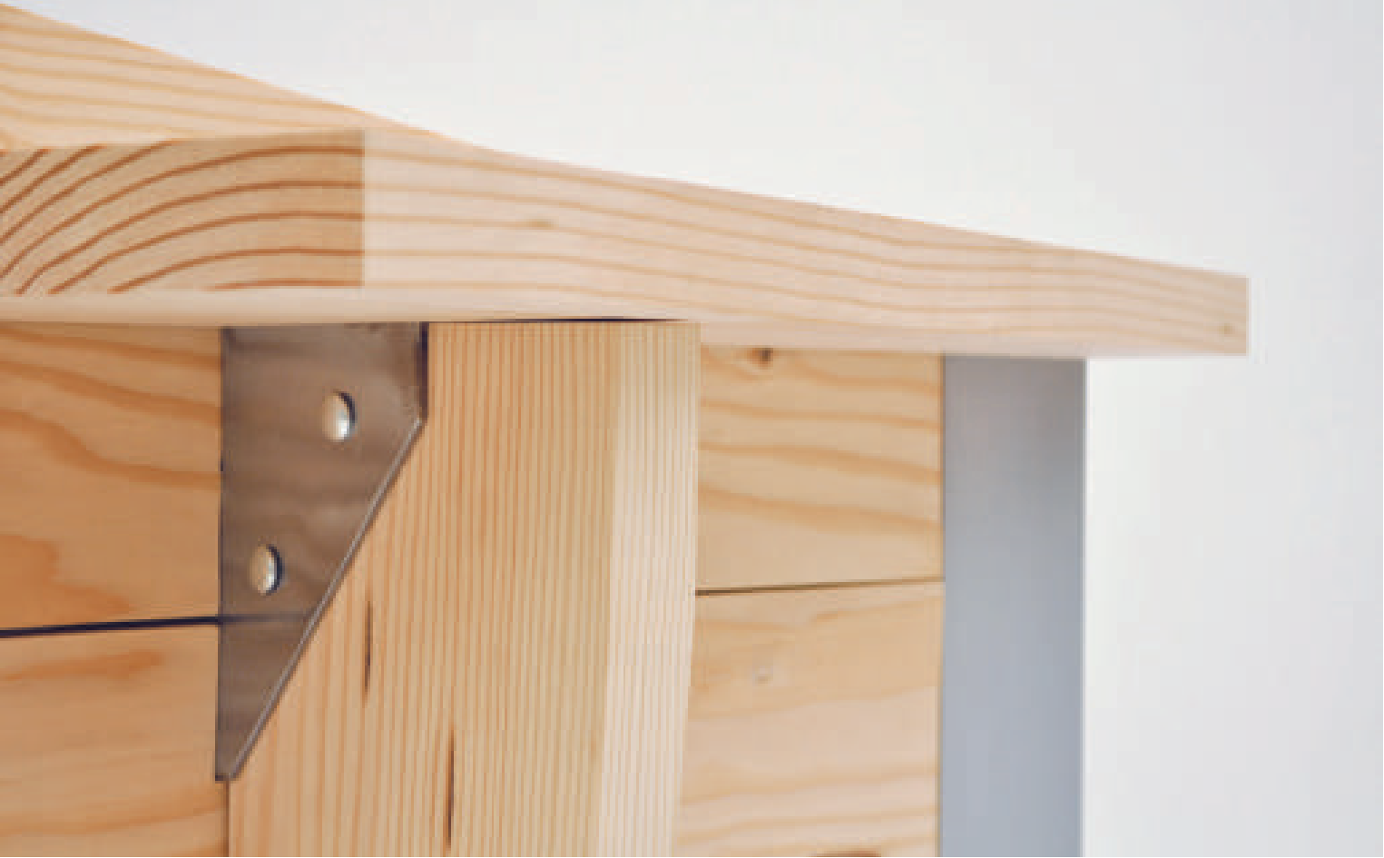
Optional seat - 1/8" Steel brackets are pre-riveted onto support legs, then slot into seat channels.
