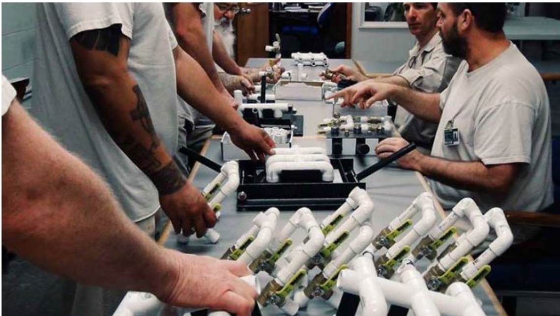
Incarcerated individuals who work in the Washington State Penitentiary's Sustainable Practices Lab assemble SafeTap water filtration systems (Washington State Department of Corrections photo).
