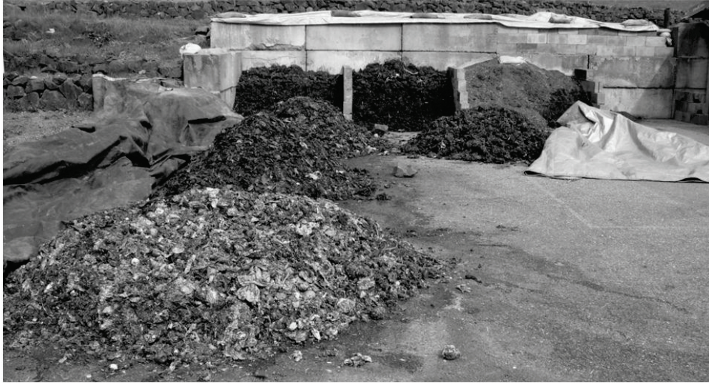
Figure 2. Outdoor piles. Foreground piles are still composting, while those in the bays are finished compost ready for screening. Every three days piles are “turned”. Turning is accomplished by moving outside edges of a pile to a new location. The outside material becomes the center of the moved pile. The center of the old pile becomes the top and edges of the new pile. Background piles are ready for sifting and may sit until time for this task is available.
