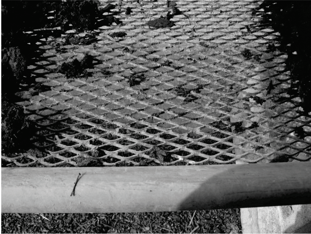
Figure 4. Sifter constructed of \frac{1}{4} in expanded metal in a frame of 3 in metal pipe.
