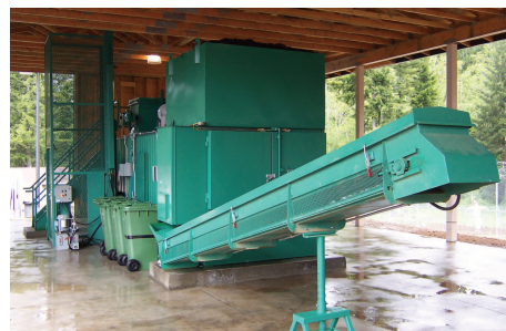
Larch Corrections Center is located in a remote area at a former forest camp. Savings from transportation costs and avoided tipping fees made the case for developing on-site composting capacity (Wright Environmental system shown above).
