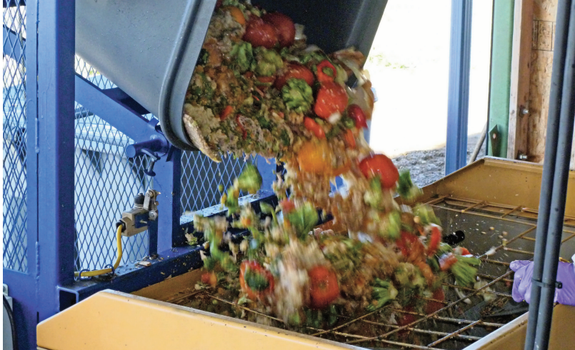
A cart lifter is used to unload food waste into the hopper of the mixer of a new in-vessel composter installed at Cedar Creek Corrections Center.
